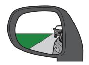
Adjust tilt to have the horizon appear in the center of the mirror. And, adjust the viewing angle to see a slight amount of the vehicle, which is essential to detect other traffic.
